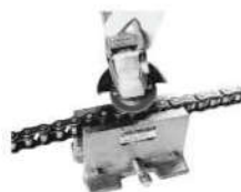
Figure 3: Grinding Down Pin Ends
