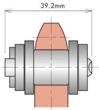
RS Sprocket (for double strand chains)
