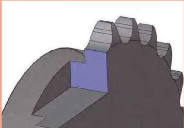
Cross-section observation of tooth hardened layer depth
