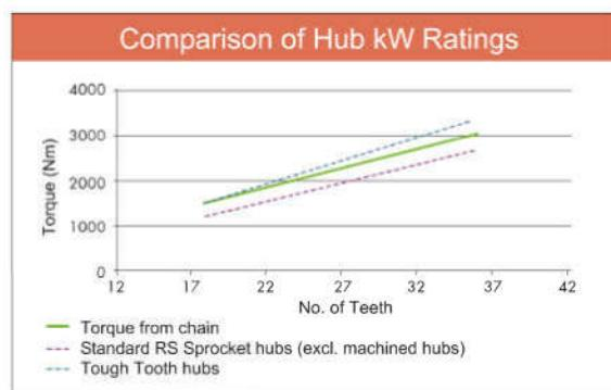
Note: 1. Torque is calculated from the keyway allowable surface pressure using a JIS parallel key at the maximum shaft hub diameter.
