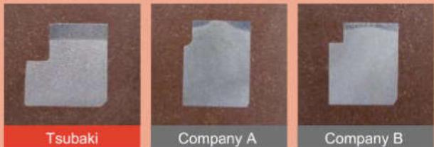
Comparison of Tooth Profile Wear When Tested under Load
