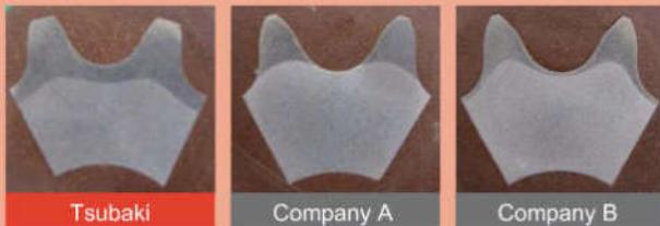
Comparison of Tooth Hardness and Hardened Layer Depth
