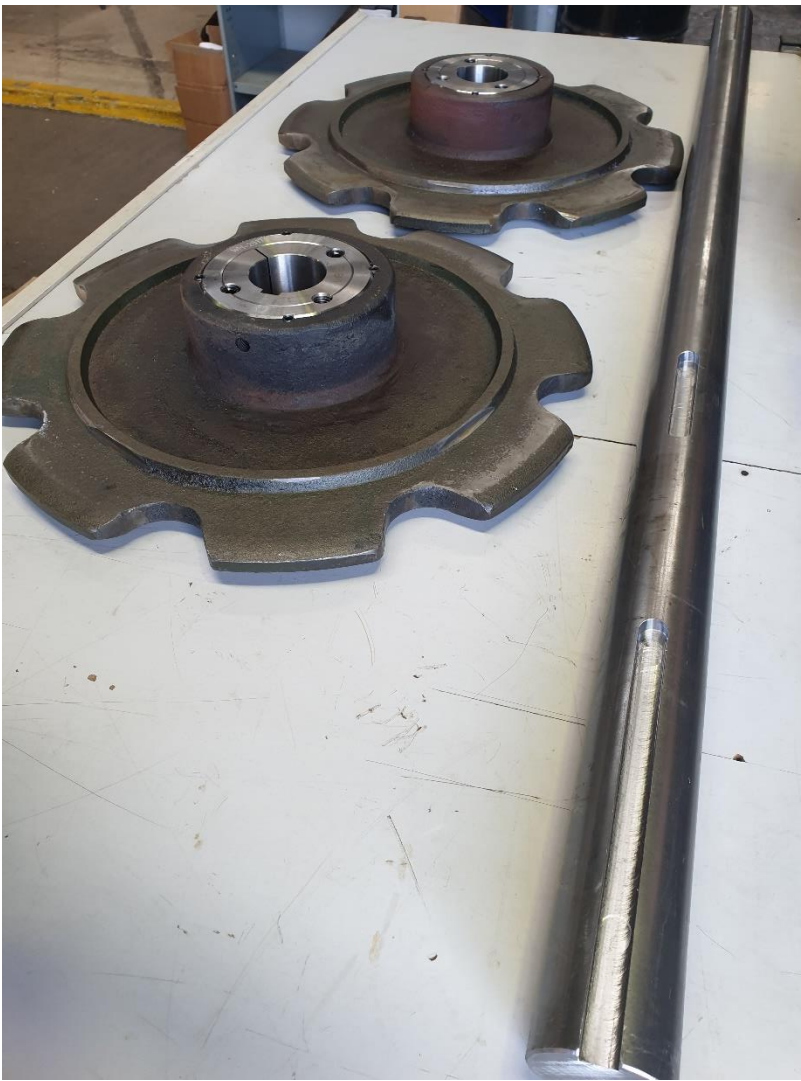
New drive shaft and old cast sprockets with weld-in hubs
