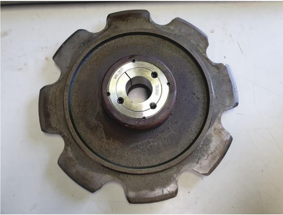
Close up look of Cast Iron sprocket with weld-in hubs
